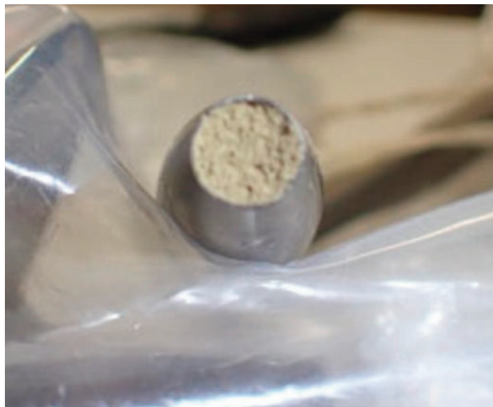
Figure 4. Larvae of Wall Mason Wasp in a pitot tube.
