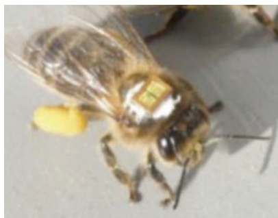
Short range RFID i.d. tag on Apis mellifera worker.
